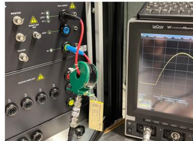
Short circuit current with current probe
