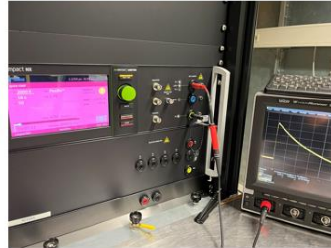
Open circuit voltage with HV-Probe
