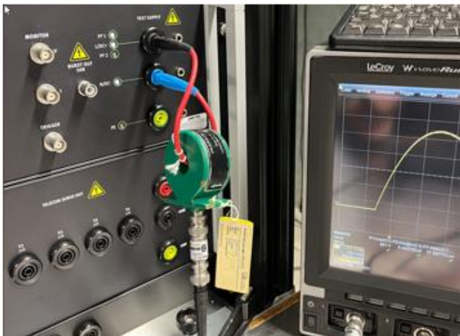
Short circuit current with current probe
