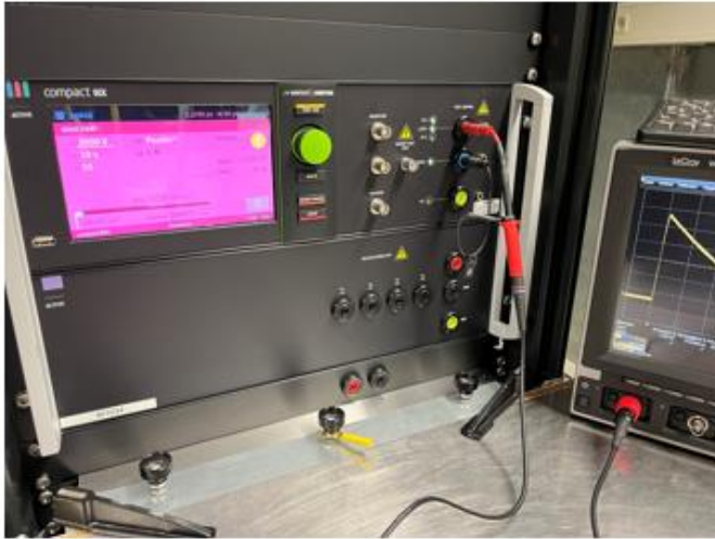
Open circuit voltage with HV-Probe
